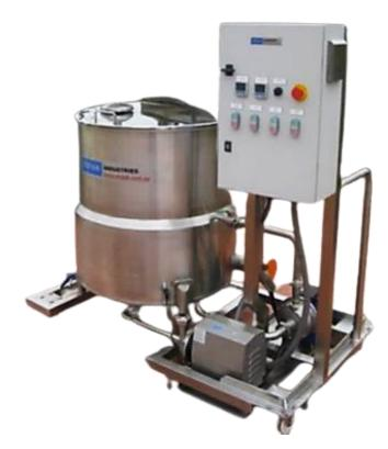
The standard MP series batch designed and constructed to pasteurizers Food are safe Australia's guidelines and compliance. All product contact parts are in SS316 food grade construction. The agitator is designed to mix powder and other ingredients. With optional Touch screen system, it is also suitable for pasteurizing Milk for bottling, cheese making and yoghurt making with dedicated control settings
