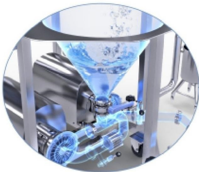
Cleaning liquid is poured into the hopper
