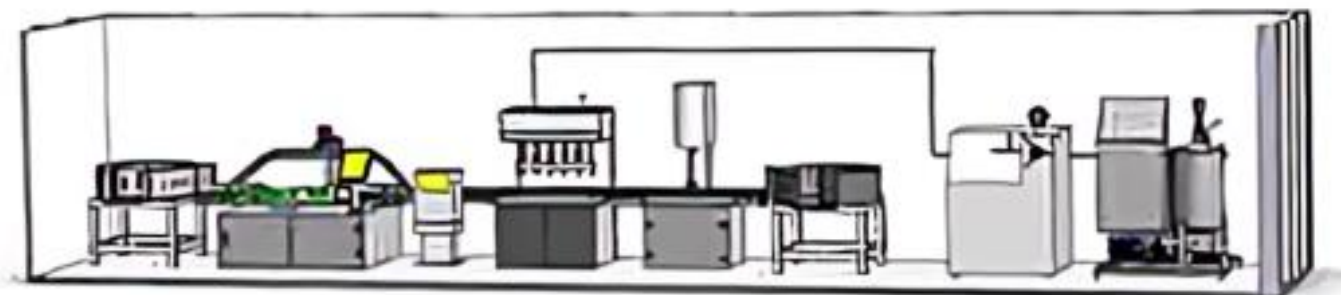
PASTEURISER CONTAINER LAY OUT
