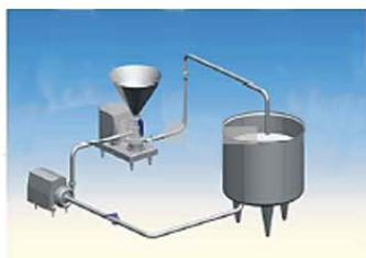
Typical Application 2: Increasing a centrifugal pump between Mixer and make-up tank is in order to feed mixer expected, this configuration can handle relatively high solid content of solution, high-speed liquid through the centrifugal accelerates solution processing of dry powder. Mainly used in the processing of final solution with solids content of 25% or less.
