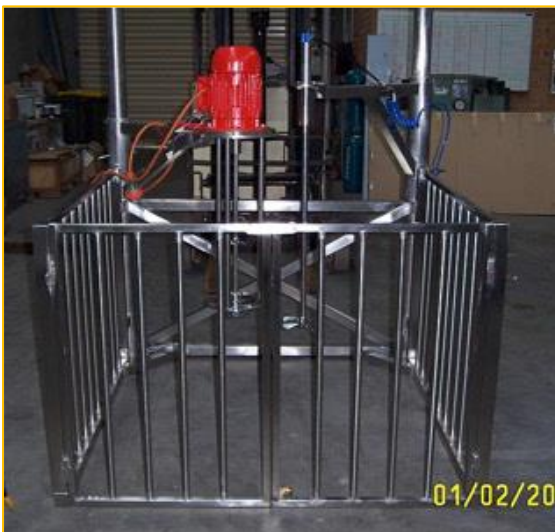
MIXER WITH PNEUMATIC LIFTS & SAFETY GATE
