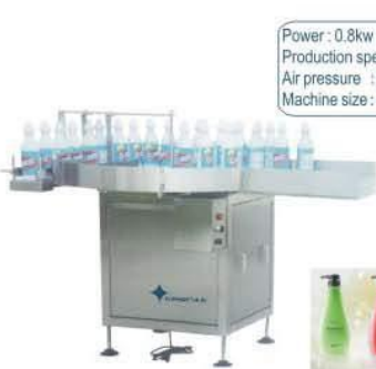
Rotating working table-infeeder bottle dia:30-100mm round,speed:7000b/h
